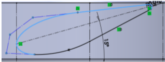
Figure 8. Screenshot from SolidWorks showing angle of attack
