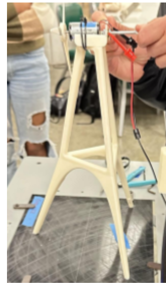
Figure 5. Attaching the motor to the wind turbine assembly before testing
