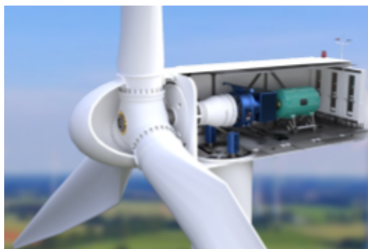
Figure 2. Inside of a wind turbine generator housing
